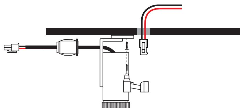
Fasten the fixture by screwing the installation plate to the ceiling.
