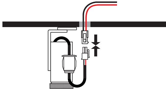
Connect the lights with the cable harness, make sure the power is turned off. The cabling can be extended up to 20 m. After this, switch on power to check that all fixtures are working properly.
