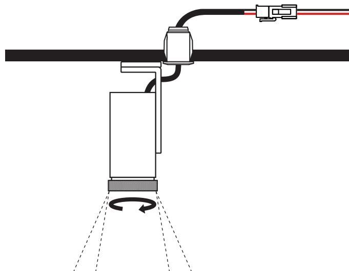
The beam angle may be adjusted by twisting the edge of the fixture.
