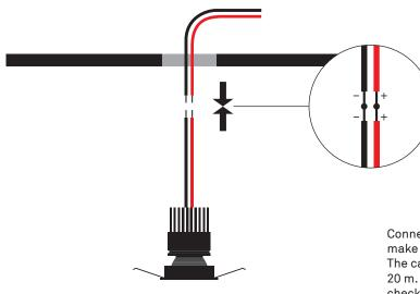
Connect the lights with the cables, make sure the power is turned off. The cabling can be extended up to 20 m. After this, switch on power to check that all fixtures are working properly.
