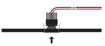
Lastly, push the Saas HD 60 Pivot into the drilled holes.
