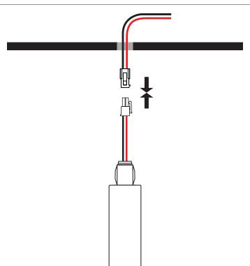
Connect the lights with the cable harness, make sure the power is turned off. The cabling can be extended up to 20 m. After this, switch on power to check that all fixtures are working properly.
