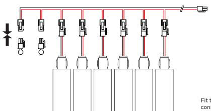
Fit the **saas loop** on all the connectors that are not in use on the cable harness.
