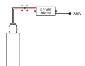
Connection scheme with several fixtures (series connection):
