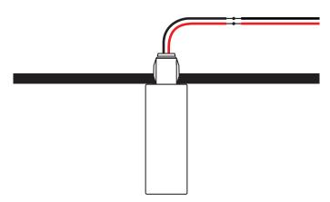
Lastly, push the led-lights into the drilled holes. The fittings are installed in the drilled holes using the installation springs.
