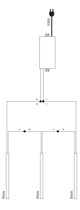
The luminaire connection should be made by a licensed electrician and in accordance with local regulations. Make sure that the power is off before installation or maintenance.
